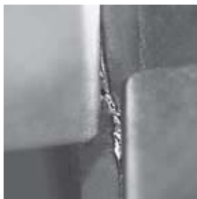
Resharpened tool (ReTool®) after 480 min. operating time
