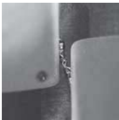
A new tool after 480 min. operating time
