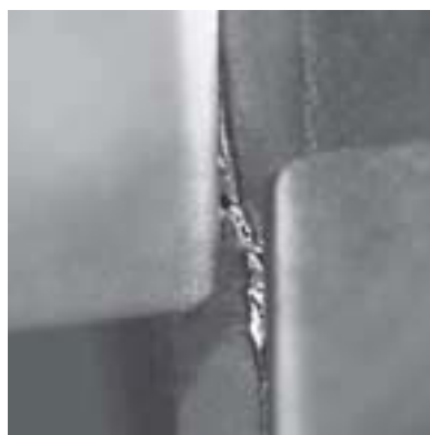
Resharpened tool (ReTool®) after 480 min. operating time
