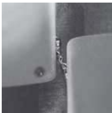
A new tool after 480 min. operating time
